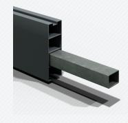
The rods are manufactured from steel tube 40mm x 30mm, manufactured to EN 10255:2004 and zinc plated to ASTM B633, ISO 2081.
